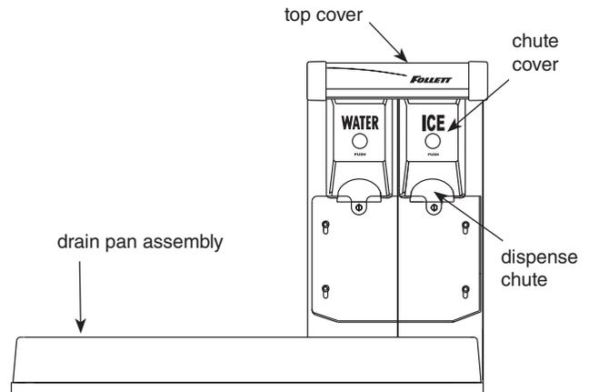
Fig. 2 – Top View, Dispense Assembly, Right Hand Unit
