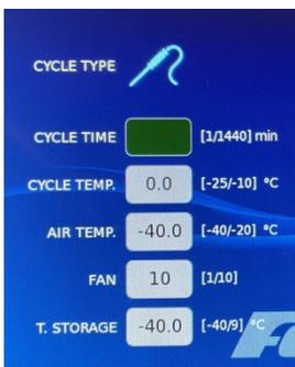
During a Temperature cycle (Needle Probe icon in the *CYCLE TYPE* tab), the multi-core needle probe of the unit must be inserted into a simulation bag. The unit will run the cycle, pulling down and holding the temperature inside the cabinet at the desired temperature as set in the “*AIR TEMP.*” tab until all of the 4 cores of the needle probe read the target temperature set in the “*CYCLE TEMP.*” tab.
