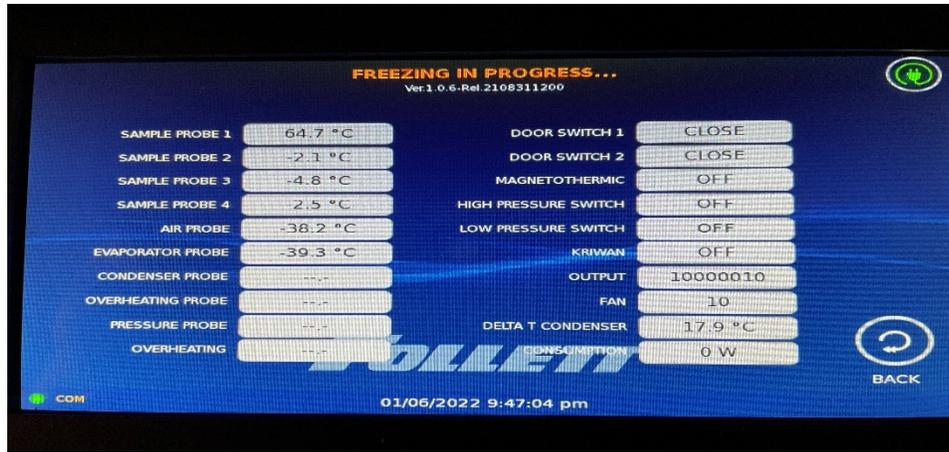
The *Input/Output* menu allows you to check all input signals, such as Temperature Sensors, Door Switch status, and Outputs such as Relays status. (Outputs shown below)
