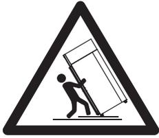
**TIP OVER HAZARD.** This unit is top heavy and tips easily when not completely installed. To avoid a hazard due to instability of the unit, it must be installed using the anti-tip brackets according to the instructions.
