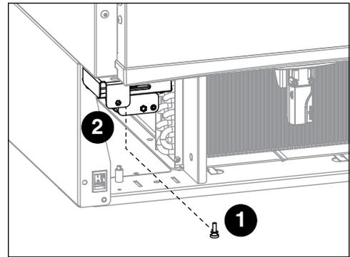
5. Pull control module forward 1 inch, rotate left as per Fig. 7, and continue to pull the control module forward.
