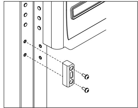
17. Support door and remove screws attaching hinge to refrigerator cabinet and remove the door (**Fig. 13**).
