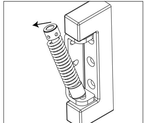
16. Remove screws and latch from refrigerator cabinet and the lock from the door (**Fig. 12**).
