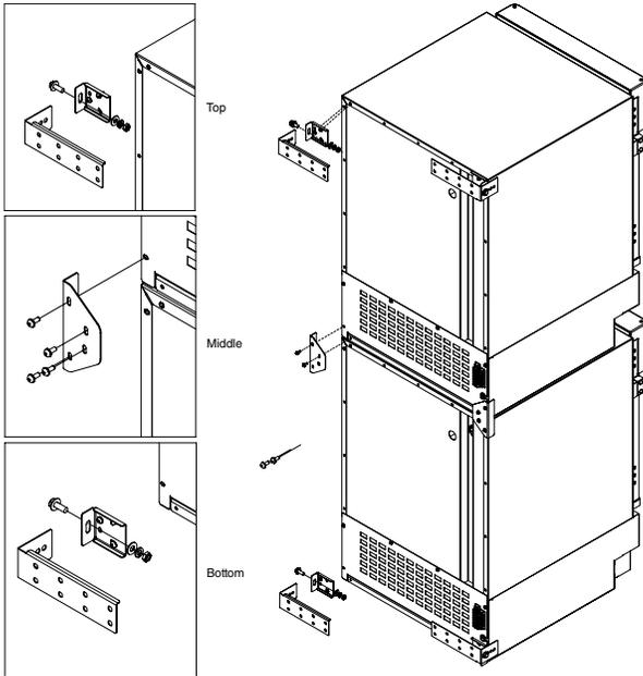
**Seismic bracket for undercounters**
