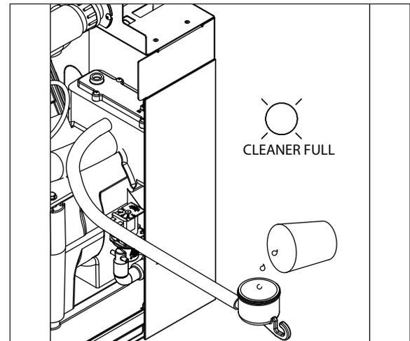
5. Replace cover on cleaner cup. Machine will clean, then flush 3 times in approximately 15 minutes. Wait until machine restarts.
