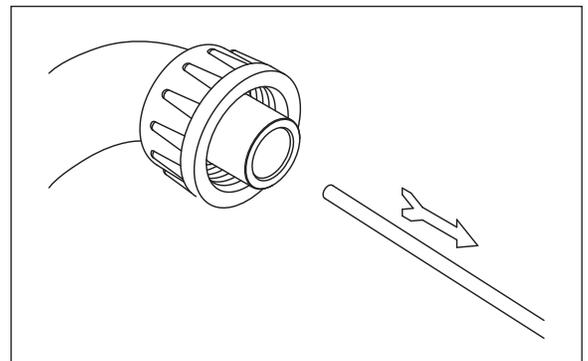
11. Reconnect coupling. Press power switch ON. Ice pushes SaniSponge cleaning sponges through ice transport tube.
