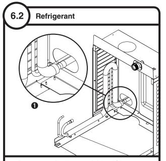
Braze supplied expandable refrigerant lines in place •
