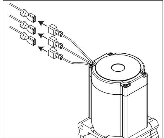
12. Remove gear motor:
