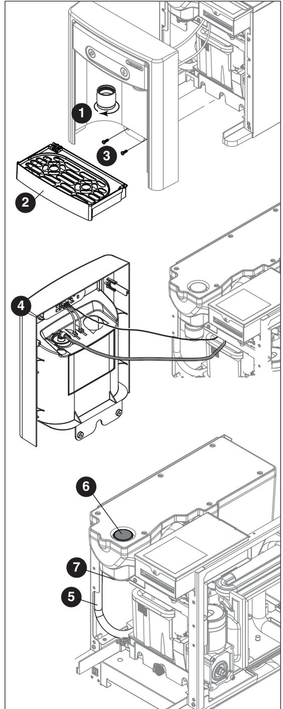
11. Locate the storage bin drain tube pinch clamp (**Fig. 10**) and engage (close).
