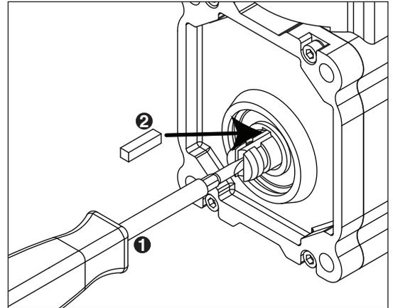
13. Install spacer, ensure that key is captured in slot (**Fig. 26.1**).
