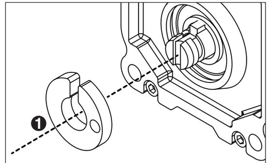
14. Insert screwdriver into groove of auger shaft and pry shaft outwards (**Fig. 27.1**).
