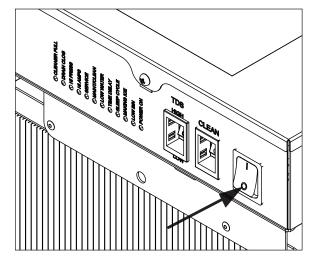
6. To clean/sanitize ice transport tube – Press power switch OFF
