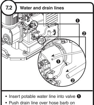
Push drain line over hose barb of back of evaporator mount 2
