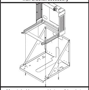
Mount docking assembly to wall bracket accessory
