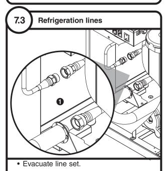
Connect self-sealing liquid and suction line fittings
