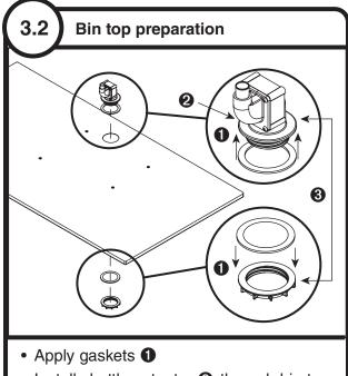
Install shuttle actuator 2 through bin top and secure with locking nut 3
