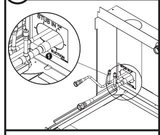
Braze supplied quick-connect lines onto stub-ins 1.
