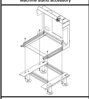
• Mount docking assembly to machine stand accessory
