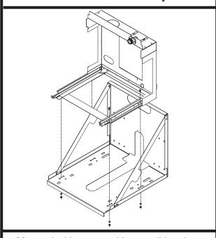
Mount docking assembly to wall bracket accessory
