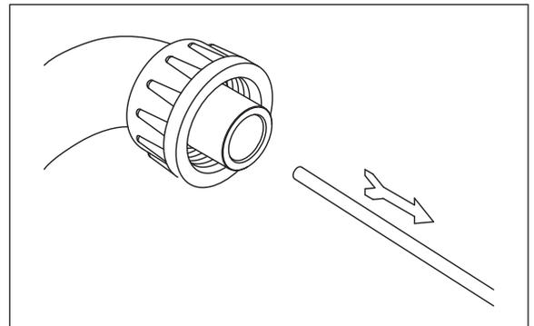
12. Reconnect coupling. Press power switch ON. Ice pushes SaniSponge cleaning sponges through ice transport tube.
