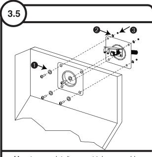
Mount cover plate/transport tube assembly on outside of dispenser using screws, flat washers 1, lock washers 2 and nuts provided 3
