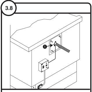
Insert bin thermostat capillary tube through hole in gasket as indicated
