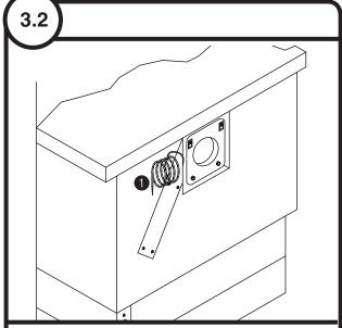
Coil capillary tube and secure away from bin fill opening 1
