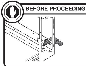
Prior to installing the louvered docking assembly, ensure that the drain fitting is oriented (right or left) correctly for your installation. An optional straight drain fitting is also supplied. You may need to remove the back panel of the docking assembly in order to re-orient or change the drain fitting. Replace back panel prior to mounting the docking assembly.
