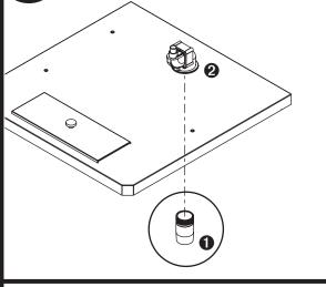
• Screw 4" (102mm) extension 1 into bottom of shuttle actuator 2
