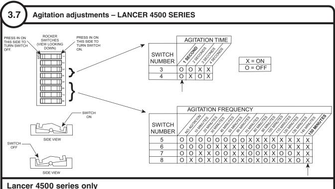
Adjust the agitation time to 1 second, and the agitation frequency to 150 minutes. See Lancer
