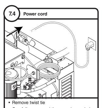
Carefully pass cord thru opening and plug into wall outlet
