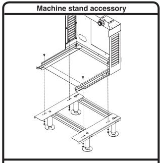
Mount louvered docking assembly to machine stand accessory
