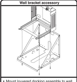
· Mount louvered docking assembly to wall bracket accessory
