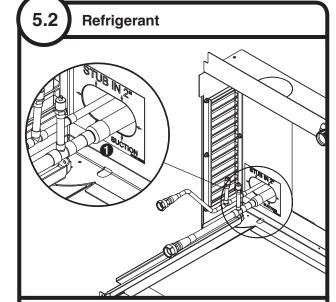
• Braze supplied quick-connect lines onto stub-ins 1.
