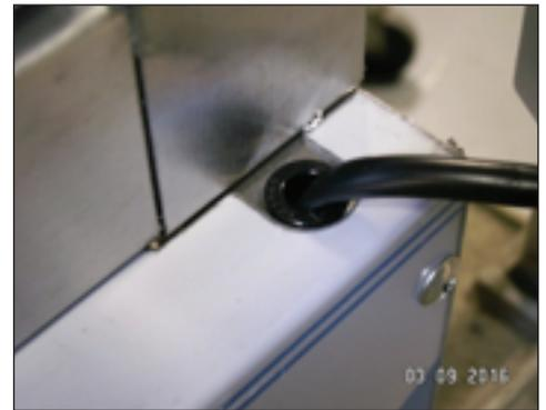
10. Remove the screw from the white strap on the hinge side of the wire channel (Carefully remove the control wire from the channel ensuring the insulation jacket does not tear.) Route through channel to opposite side of door. Reinstall the wire and strap on the opposite side of the door **(Fig. 10).**
