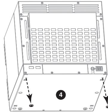
5. Remove the six screws securing the lower vent cover on the REF. For REF1, also remove and discard the two screws located on the bottom sides of the upper vent cover. *Do not discard vent cover.*
