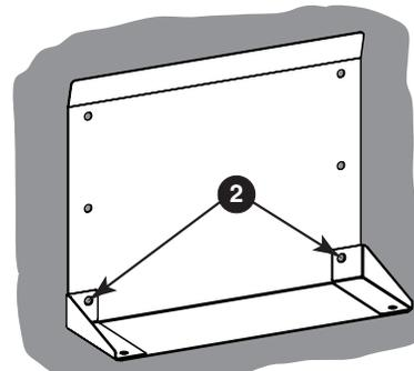
3. Tilt REF forward (not more than 30 degrees) and verify that both 5/16" speed nuts, located adjacent to the rear feet, are still installed.
