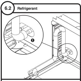
• Braze supplied expandable refrigerant lines in place **1**
