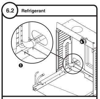
Braze supplied expandable refrigerant lines in place •
