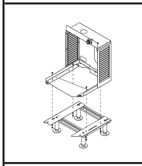
Mount louvered docking assembly to machine stand accessory
