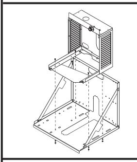
Mount louvered docking assembly to wall bracket accessory
