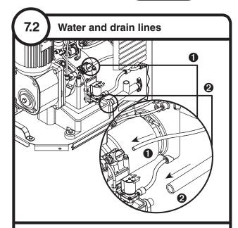
Insert potable water line into valve 1
