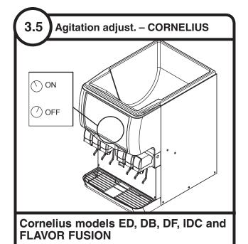
Adjust the agitation timer located on the Cornelius PC board to 1 second on, 1 hour off. **Note:** See
