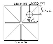
Locate hole position 5" (127 mm) from back and right of dispenser top
