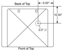
Locate hole position 9" (254 mm) from back and 9" (229 mm) from right of dispenser top
