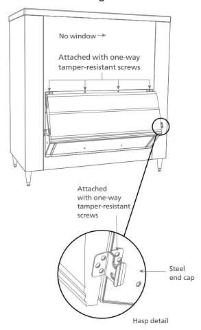
Models listed are compatible with the correctional facility package. Specify item# 00917054 in addition to desired ice storage bin or dispensing system.
