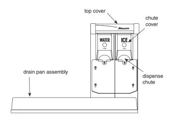
Fig. 2 - Top View, Dispense Assembly, Right Hand Unit
