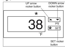
The controller is pre-programmed with a 34 F set point which provides a compressor cut-in at 38 F and cut-out at 34 F. This may not meet your specific application needs. For example, many pharmaceutical manufacturers recommend that their refrigerated medications be stored between 36 F and 46 F. Instructions for changing the set point are found below.
