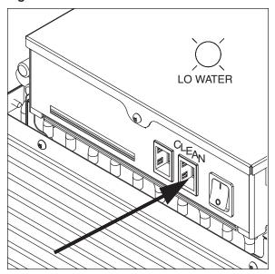
Mix 1 gallon 120 F (49 C) water and 1.6 ounces (48ml) NU-CALGON IMS-II or IMS-III SANITIZER. Fill until HI WATER light comes on (Fig. 5).
