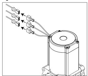
**12.** Remove gear motor:
