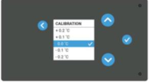
**WARNING:** Changing the calibration offset will change the performance of the refrigerator and cool/warm the unit to reflect the changes made. Changes should only be made to reflect the readings from a NIST calibrated thermometer.
