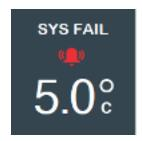
(Left Image) System Fail Alarm Indicating Loss of UI Communication with Thermal System. Dashes displayed when communication is not active and has not been for at least 2 minutes. (Right Image) Known temperature is displayed when a communication failure had occurred for at least 2 minutes but has since recovered.
