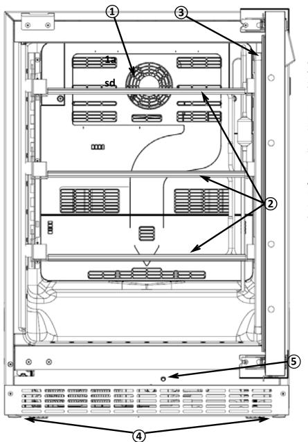
**1. Circulation fan:** Helps to keep a consistent temperature throughout the entire chamber.
