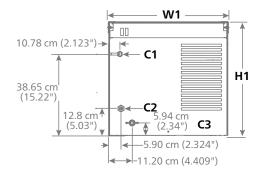
SHORT FORM SPECIFICATION: Ice machine to be Follett model number \_\_\_\_\_\_. Ice machine to produce Chewblet ice. Ice machine to have stainless steel evaporator, auger and top bearings, heavy-duty tapered roller bearing, and low-water safety circuit. NSF listed.
