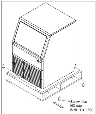
Fig. 2 - Leg Set (Freestanding) or Leveling Feet (Undercounter) Option
