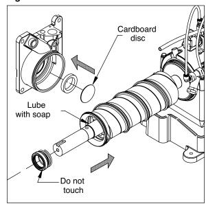
5. Reinstall main housing as shown.
